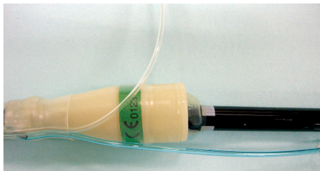
Fig. 3 Thick white line indicating the 155-cm marking on the endoscope.
